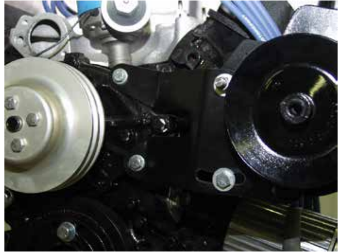
This photo shows the pump adjusting bracket and pump mounted to the water pump and head.
